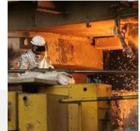
Fig 3 Operator lancing the taphole
