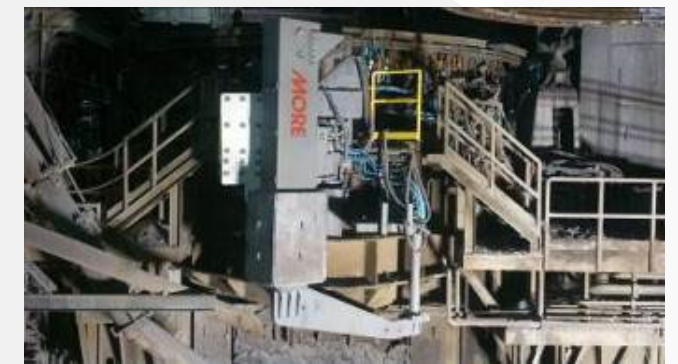
Fig 3 STROP in operation on an EAF in Mexico
