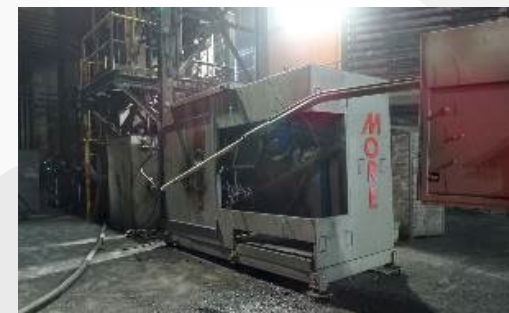
Fig 7 Automatic cardboard sample tube changer
